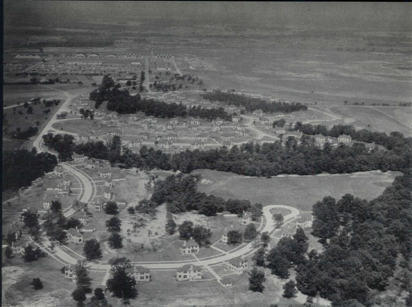
Air view of Maxwell Field, Alabama. There a slightly rolling and partly wooded area was used to advantage in an informal layout of Officers' Quarters, almost all of which were built at the same time.
