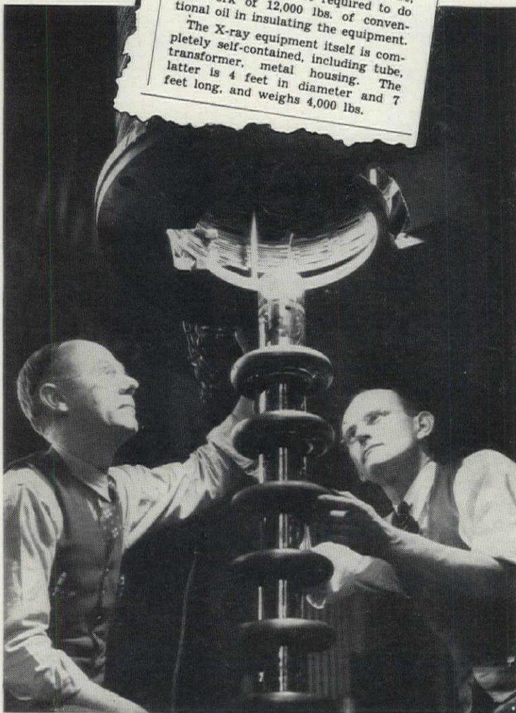
G-E workers assembling the new million-volt X-ray therapy unit.
