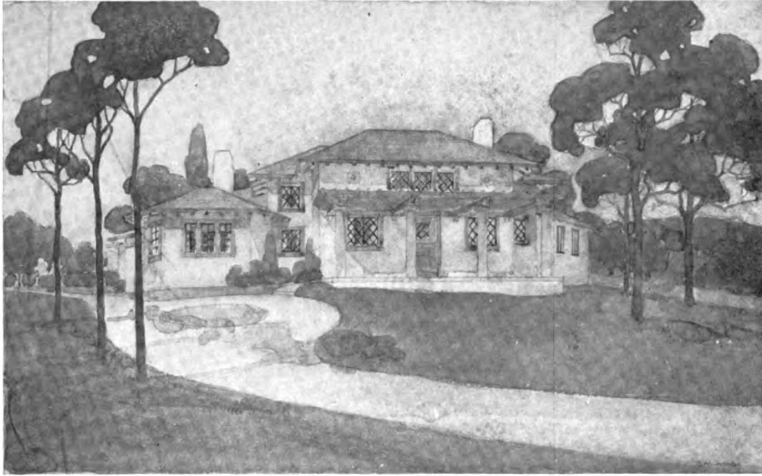
VIEW OF A COTTAGE BUILT IN THE SUBURBS OF NEW YORK FOR $7,400 Sullivan W. Jones, Architect Built of cinder concrete mixed in the proportion of 7 to 1 Cement Age
