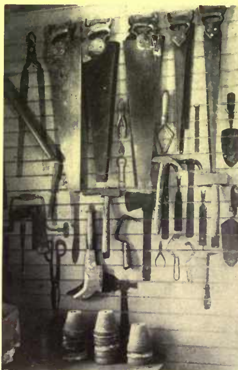
The shape of every tool is painted on the wall, so that each implement has its particular place
