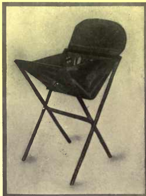
This handy little work stand folds up somewhat in the manner of a camp stool
