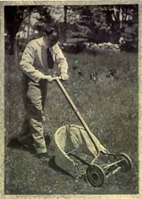
A canvas attachment to the lawn mower will save the grass clippings for use as mulch
