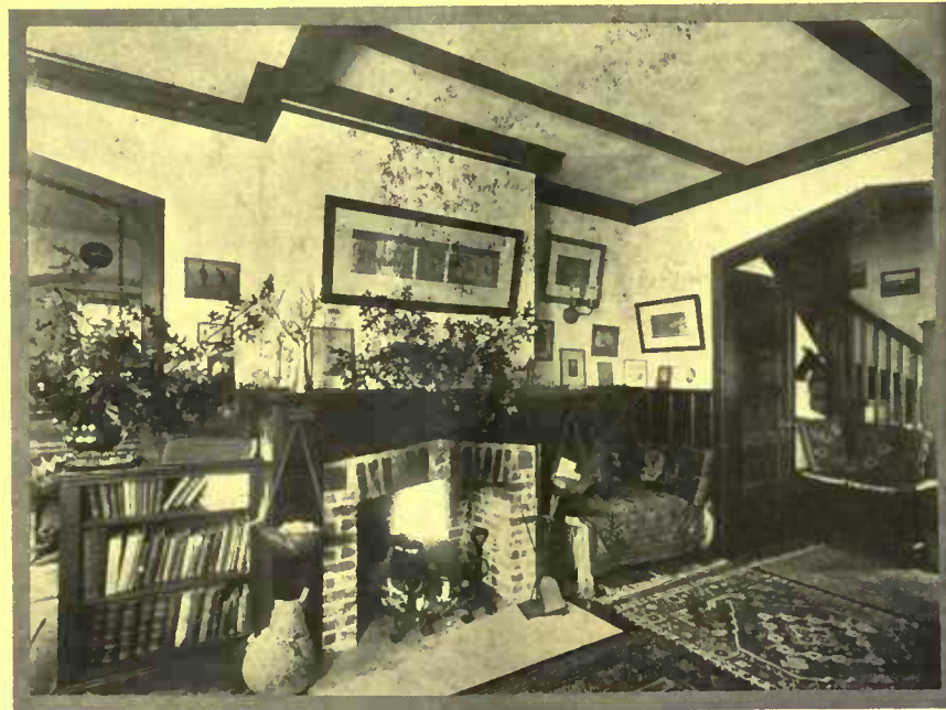
The fireplace is flanked by a built-in seat, balanced on the other side by a bookcase, both made possible by the deep chimney.
