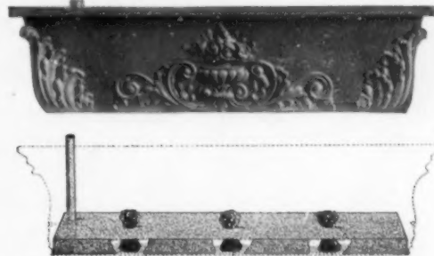
The tube in the left hand corner extends upward for the purpose of pouring water into the reservoir in bottom which supplies moisture to the roots of plants through sponges and holds sufficient water to last 10 to 20 days.
