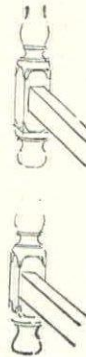
Flush construction shows the face of the joint smooth where the two pieces meet, a feature of fine furniture. The stretcher above is set back from the face, a slovenly method of joining such pieces
