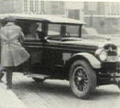
Illustrating the rigidity of the chassis of The NEW STUTZ Safety Chassis. With one wheel on the curb, the doors open and close without sticking.
