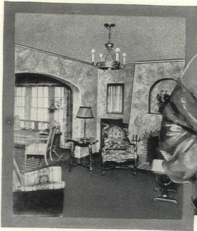
Rough-texture effect over Gypsolite wallboard, in the Ashenhurst house, Chicago, America's best insulated home.
