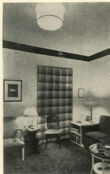
LEFT: Ceiling fixtures have assumed a new and much more pleasing form, combining the best features of direct and indirect lighting
