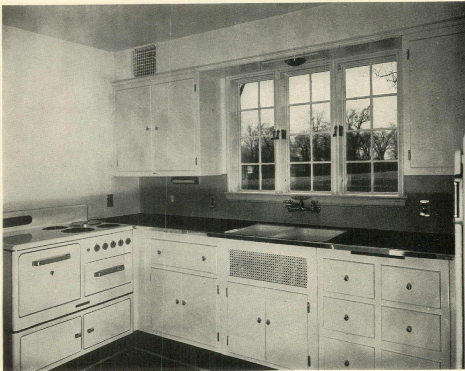
A practical plan for "turning the corner" with equipment. Note the exhaust fan in the furred ceiling
