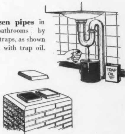
Fireplaces in unused rooms should have their flues sealed with a metal cap to prevent seepage of moisture. Warm rooms keep chimneys dry.
