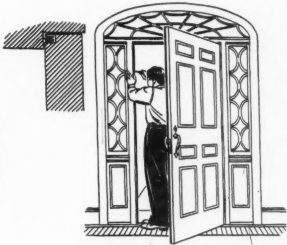
A hole in an outer wall large enough to crawl through would soon chill a house. Actually the total of all cracks around windows and doors often equals this. Apply weatherstrip throughout.
