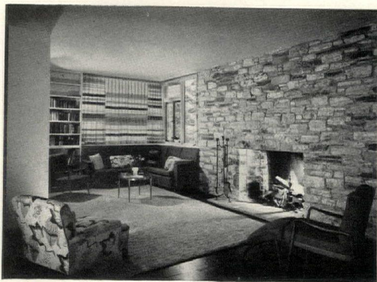
The plaster ceiling is the source of heat.
