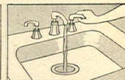
Turning on cold water automatically starts Disposall motor.
