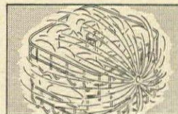
Water swirls in around safely racked dishes to rinse and warm them.
