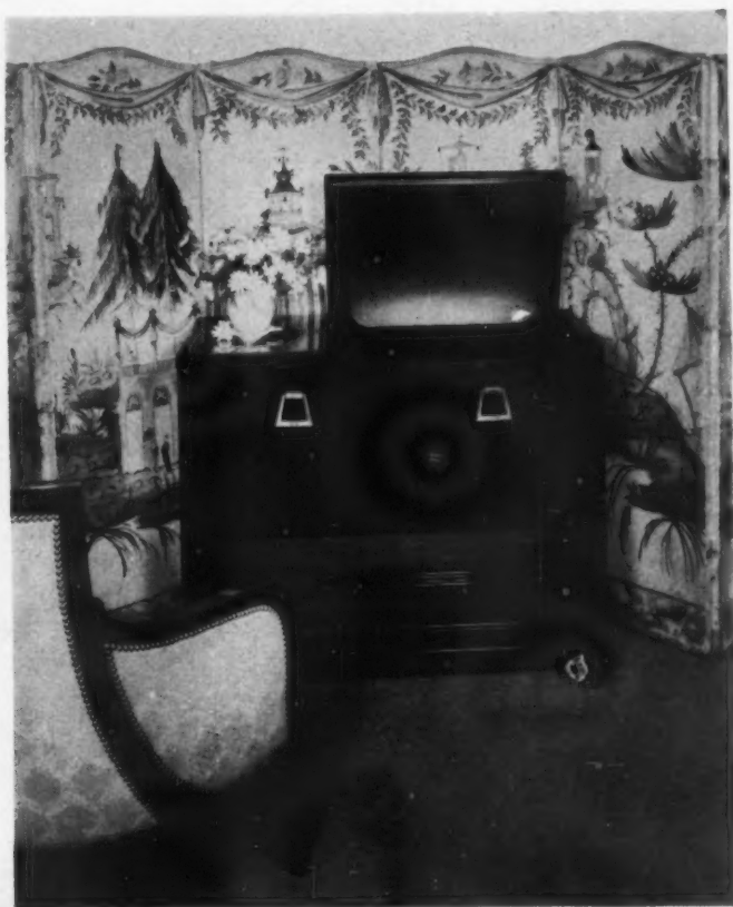
PHILCO "Projection Receiver" in a mahogany console, reflects the image on a screen 20" x 15" from a 4" tube. It is $795 at Macy's, N. Y.
