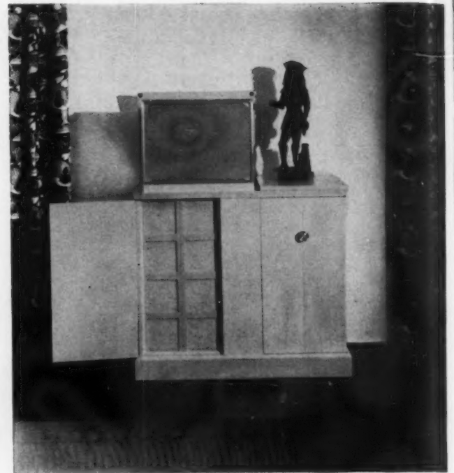
UNITED STATES TELEVISION "Hamilton" is a combination of television, radio and record player in a bleached mahogany cabinet. The image is magnified to 22" x 16" from a 5" tube. The set costs $1795 at Wm. Knabe & Co., N. Y.
