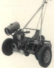
For extra large lawns, parks Toro's 27" Starlawn gives high capacity power with 2.5 HP, 4-cycle engine. Adjustable cutting height, all-steel construction, finger-tip controls take labor out of all-day mow-
