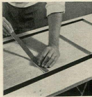
Step 2. You apply the strips to the panel 1 inch in from the edges in a trellis-like pattern.
