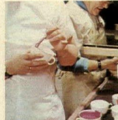
Dipping the ware in glaze and painting an extra layer on to vulnerable areas. It is then fired in the glaze oven for 7 hours at 1100C.
