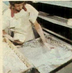
Dipping the ware in glaze and painting an extra layer on to vulnerable areas. It is then fired in the glaze oven for 7 hours at 1100C.
