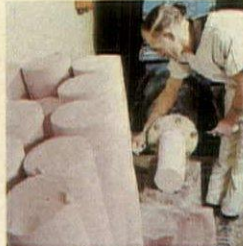
The pug mill removes air from the clay to make it pliable.
