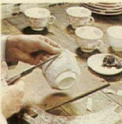
Tailoring the transfer to the shape of the cup.
