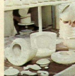
To make a teapot, liquid clay is swirled inside a mould.
