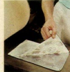
Taking a transfer print from a copper plate.
