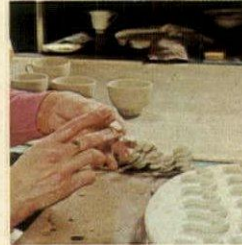
The handle and foot are attached with liquid clay so that after firing, they become one with the body.
