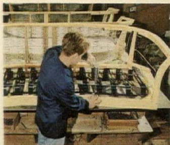
Lifetime springs are permanently attached to the solid, kiln-dried hardwood frame. Frames are double-doweled, not just glued.
