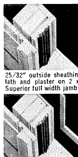
25/32" outside sheathing and dry-wall (3/4" or 1/2") inside on 2 x 4's, and "Superior" minus inside strip on jamb.
