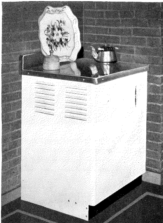
York-Shipley unit has 90,000 Btu hot water boiler plus domestic hot water coil. It must sit next to brick or insulated wall to get a chimney outlet. In Levittown houses (H & H, Feb. '52) it is in kitchen and stainless steel top provides a valuable work surface. Size: 30" x 25" x 36".
