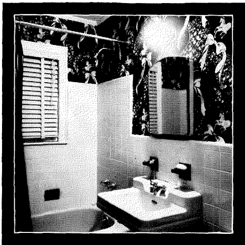
Single overhead bulb blinded persons looking into mirror. Shaving or grooming was difficult because "terrific" shadows predominated on underside of face and on neck.
