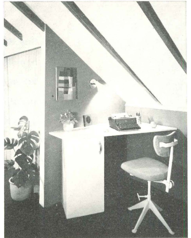
Sanded and waxed, the slender tapers of exposed beams assume a theatrical dimension in the white ceiling. A plywood sheet on a kitchen cabinet makes the work table.
