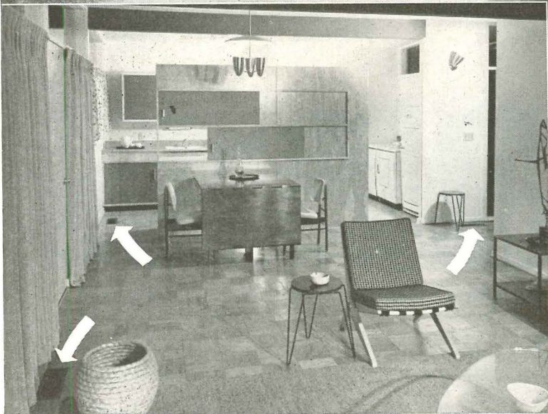
Arrows indicate outlets for conditioned air provided by a Chrysler Airtemp Furnace and a 3 H.P. Air Cooled Air Conditioner and distributed through a perimeter duct system in slab floor. Says Builder Howard C. Grubb: "I particularly like the Chrysler Airtemp cooling unit because of its flexibility. Compressor can be placed conveniently any place in house or garage."
