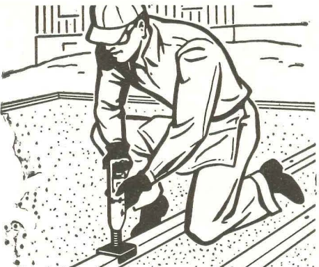
2" x 4" plates to concrete floor
