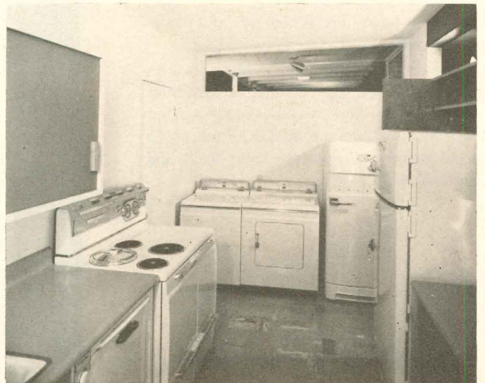
Kitchen laundries can be too crowded, and too far from bedrooms. They add to the heat, moisture and noise.
