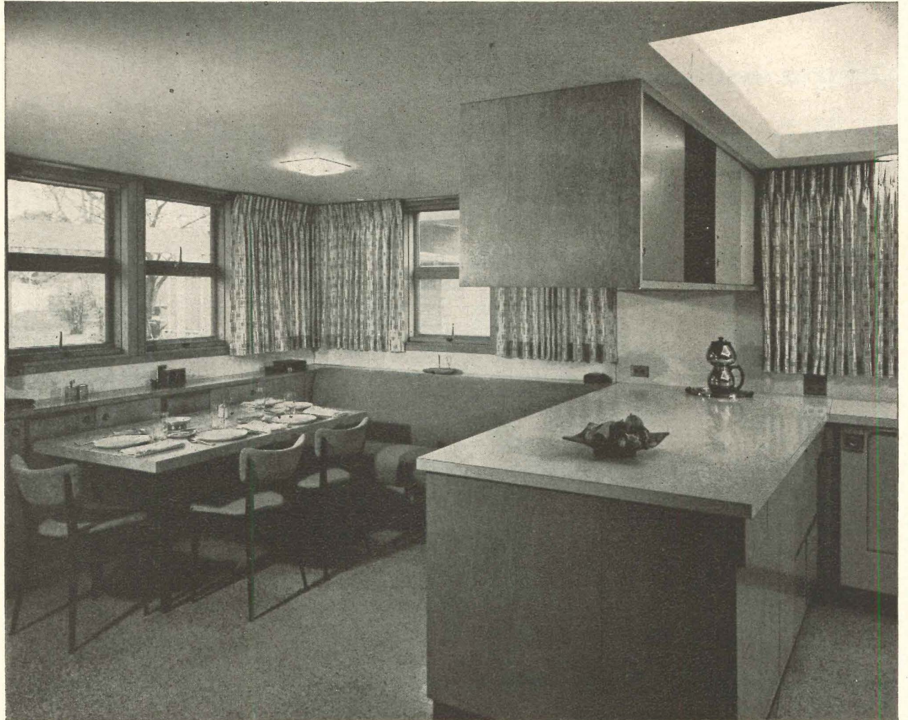
Laminated plastic counter tops resist burns and stains, come in cheerful colors
