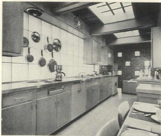
Kitchen (above), at west end of house, was photographed in natural light. With block in skylights as well as above work counter, brightness illumination ratio is 11 to 1 on a clear morning. Boyd says the ratio in most houses is 100 to 1, but should not be more than 15 to 1. (Light coming in should not be more than 15 times as bright as the natural level of indoor illumination.) Study (right) has no windows, gets at least 60 ft-c. of illumination from skylights, even on overcast day. Study's summer temperature averages 8° lower than outdoors.
