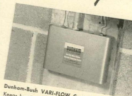
Dunham-Bush VARI-FLOW Outdoor Control Fluid-filled bulb, hidden under shield, tunes in weather changes . . . transmits temperature drop or rise to master control box.
