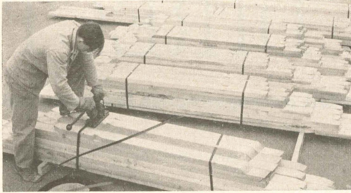
Dick Dickman: waste from shoo-cut frames makes stakes and cripples.
