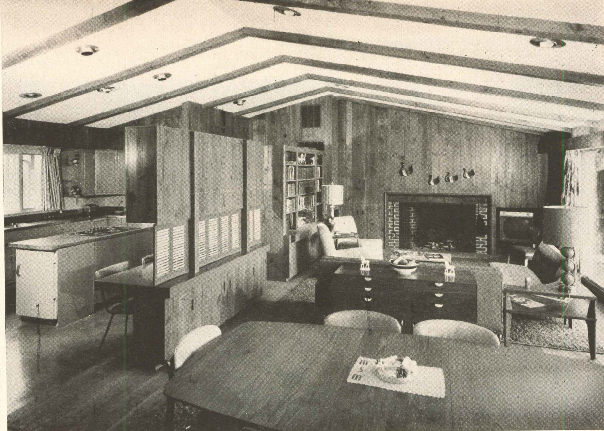
Family-room-kitchen has scissor truss ceiling. The white pine walls are from a 90-yr. old barn.
