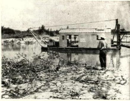
580,000 DREDGE pumps as far as 2,000'. Unit shown is made by Ellicott Machine Corp.
