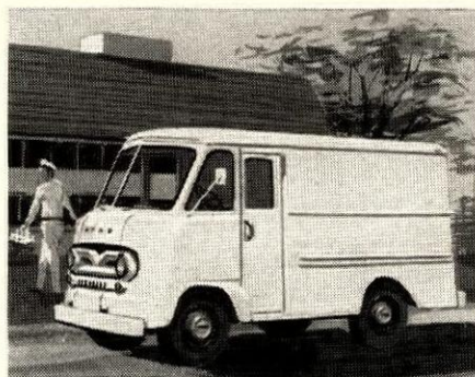
P-350 Parcel Delivery chassis with 104- and 122-in. wheelbases for 7- to 11½-ft. bodies with maximum load-space in stop-and-go service.
