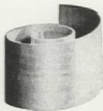
WOOD CURL is precision-cut 1 \frac{5}{8} " hardwood shaving. About 1,000 are used per 4'x8' panel.
