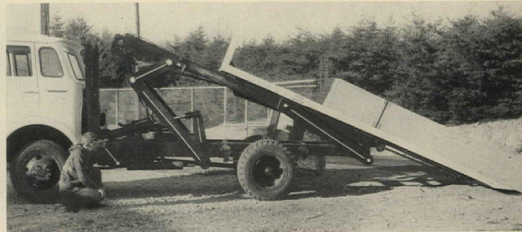
HIGH-LIFT TRUCK can carry loads up to 6,000 lb, put them on the roof (above), or slide them to the ground or into a garage (right).
