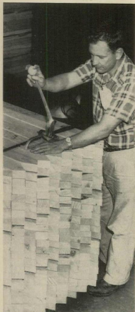
PRECUT TRUSS PARTS save local fabricators as much as $1.75 a truss. They are strapped by West Coast mill for easier shipping and more efficient handling.
