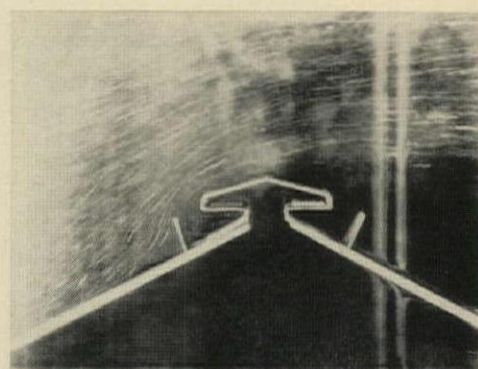
WIND-TUNNEL TEST shows how wind-driven rain or snow is deflected over the peak by vinyl baffle.
