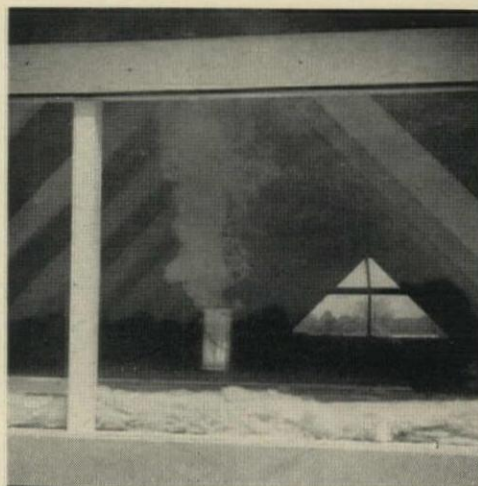
IN SMOKE TEST attic ridge vent cleared attic in 1½ min, gable-end vents took 9 min to clear.
