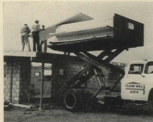
HIGH-LIFT TRUCK can carry loads up to 6,000 lb, put them on the roof (above), or slide them to the ground or into a garage (right).
