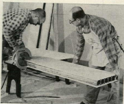
CUTTING PANELS is easy with a portable electric power saw or an ordinary hand saw.
