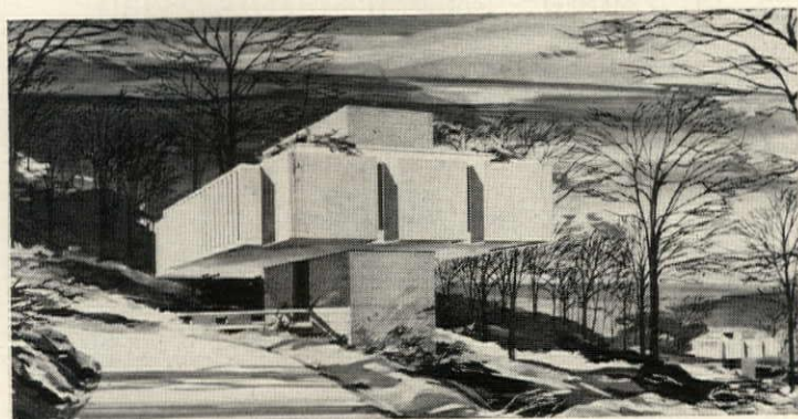
FIRST HOUSE will cantilever on steel floor beams, have a brick facade.
