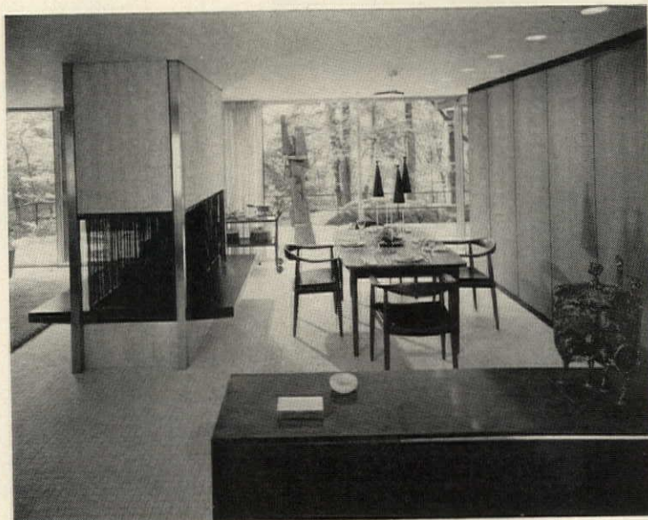
Freestanding fireplace of Travertine marble and stainless steel divides living and dining area. Hearth is black slate on reinforced concrete.
