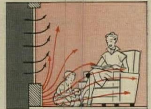
When walls and floor are warm, cold drafts are eliminated—all the space in the room is comfortably warm.
