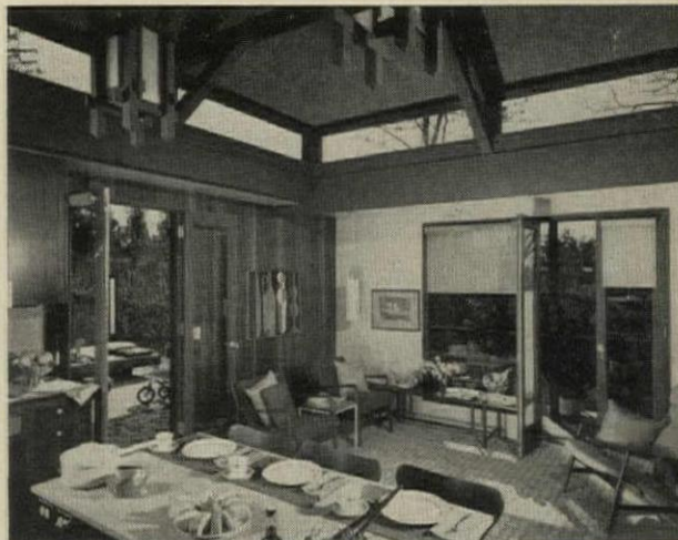
Kitchen-family room has its own pyramidal-roof, gets extra daylight from the clerestory windows above the walls on all four sides.
