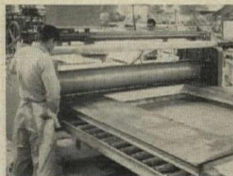
GLUE SPREADER at National Homes applies glue to sheathing (to receive aluminum siding) at a 1' per sec. rate. Cost: $6,000.
