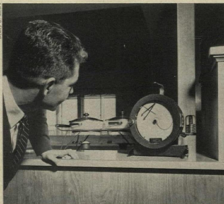
COOLING RESEARCH checked comfort and cost of 22 air conditioning systems under actual living conditions in 22 houses. Results showed that correct installation of equipment and ducts could halve operating costs, also helped establish permissible noise levels for cooling machinery.
