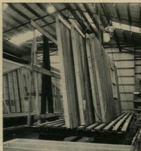
PANEL TRAILER has steel frame to support panels. Spaced-member floor locks in panels permits skirts to extend below. One-ton hoist hangs from girder.
