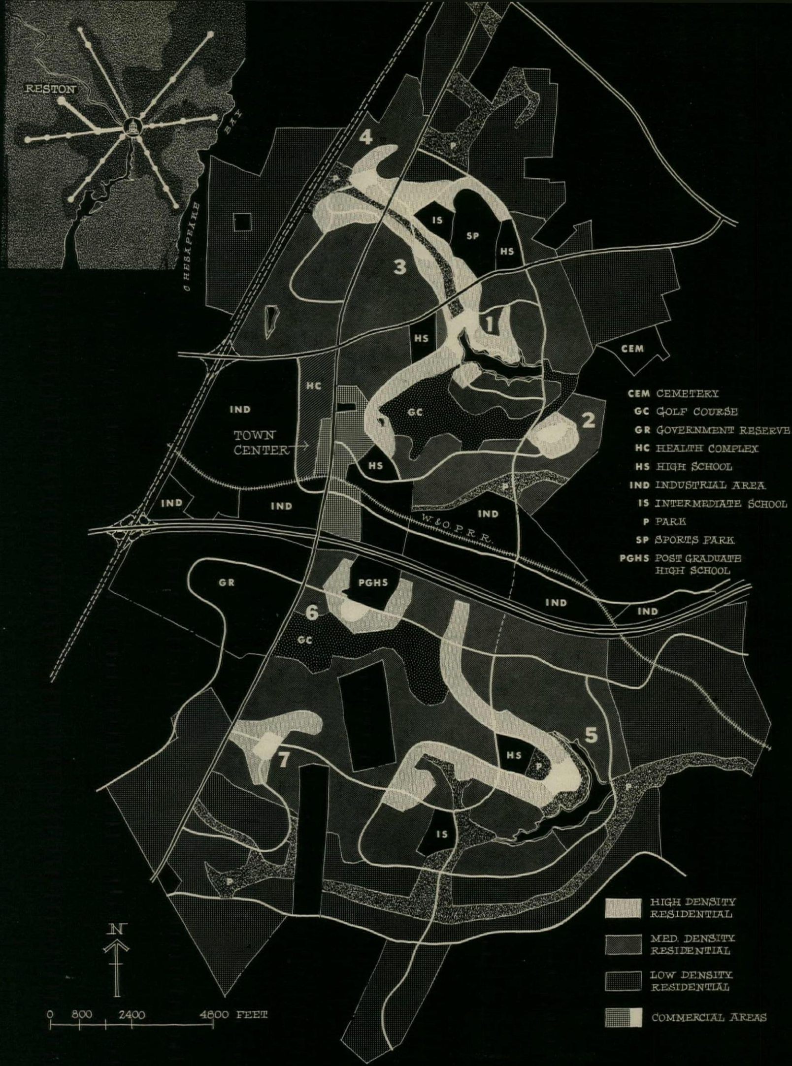
RESTON MASTER PLAN provides thorough mix of many types of units on rolling land. This was made possible by residential planned community zoning.
