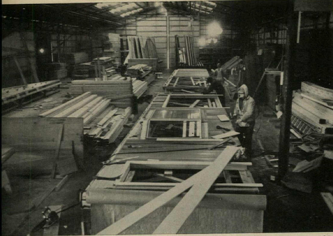
EXTERIOR WALLS are prefabricated on 80' jig table. Lumber for studs and plates is at left, sheet materials are at right. Roll in foreground is building paper. Note the wide span at far end of the factory, made possible by open-web steel bents. Doors ( rear ) are 20' high, 24' wide.
