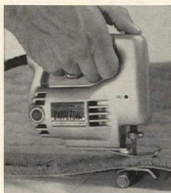
Carpet cutter can cut through any carpet and pad, cuts straight lines, curves or angles. Carpet saw weighs only four lbs., lists for less than $80 and is available from rug and linoleum dealers. Crane Cutter Co., Santa Clara, Calif. (For details check No. 23 on p. 147)
