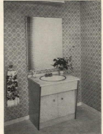
Vanities are made of particle board and high-pressure laminate. Apron, doors and toeboard are recessed. Exposed edges are capped with gold or silver aluminum trim. Standard vanities are 24", 30", 36" and 42" wide. Andy Place Prods., South Bend. (For details check No. 20 on p. 147)
