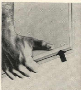
Gypsum wallboard has new beveled back edge that lets panels butt tightly together. Bevel relieves edge pressure, allowing more secure nailing. Eased edge also is less sharp, making the sheets easier to carry. Celotex, Chicago. (For details check No. 22 on p. 147)
