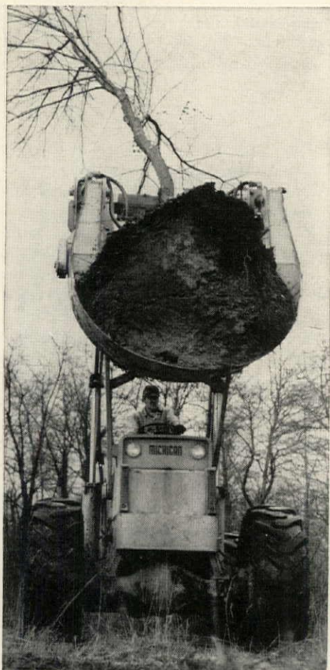
TRANSPLANTING by wheel loader is simplified by keeping tree roots cut back at nursery.
