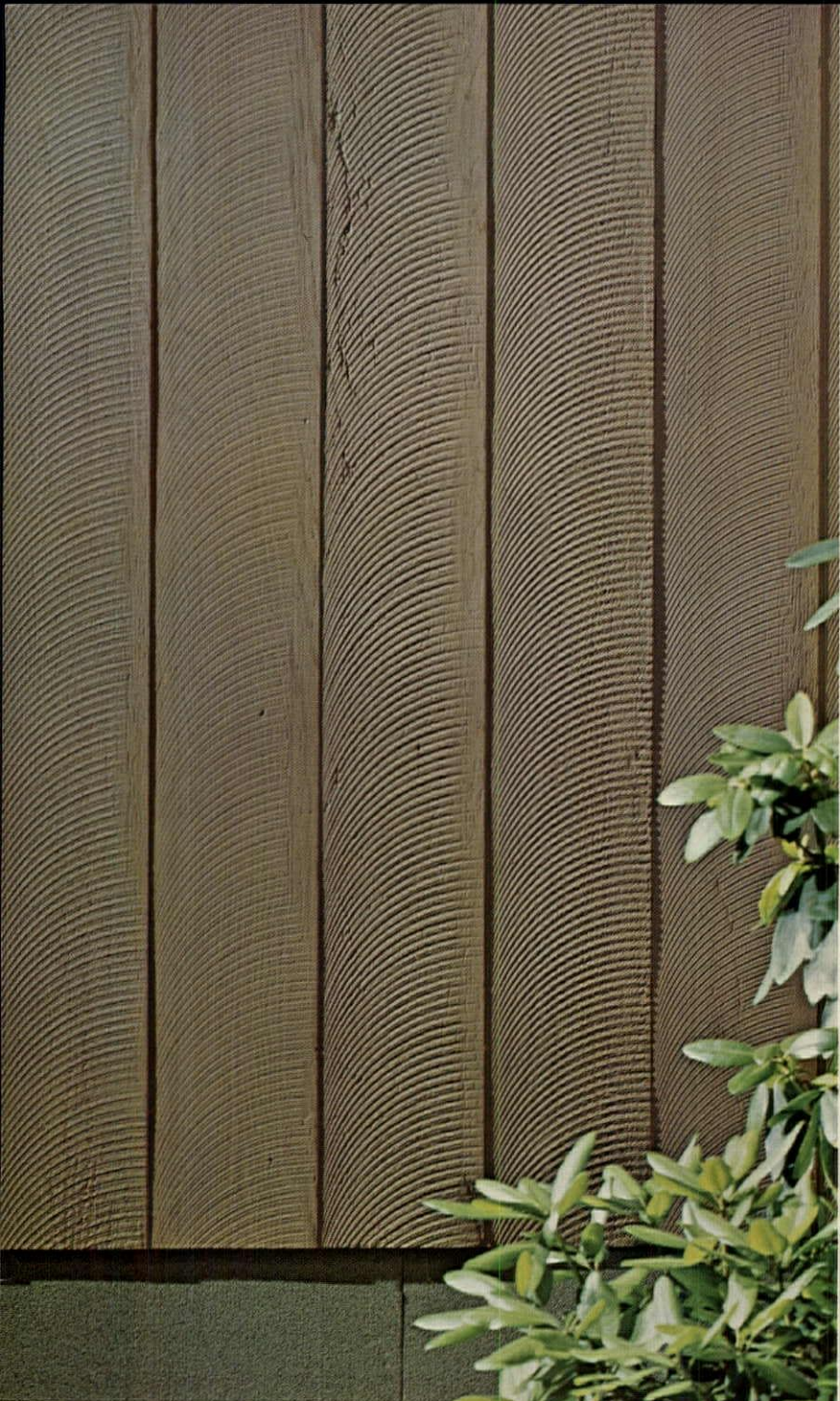
WELDWOOD PLANKTEX® SIDING —Rough-sawed sections create a lap effect with distinct shadow lines every 8". Apply it vertically, with or without battens, or horizontally for a lap-siding look. In redwood or fir.
