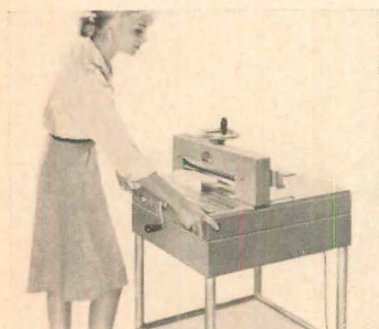
Electric paper cutter takes paper up to 21" wide and cuts over a ream at one stroke. It shuts off automatically after every cycle for safety and economy and comes with a one-piece metal stand 34½" high. Michael Lith, New York. Circle 211 on Reader Service card
