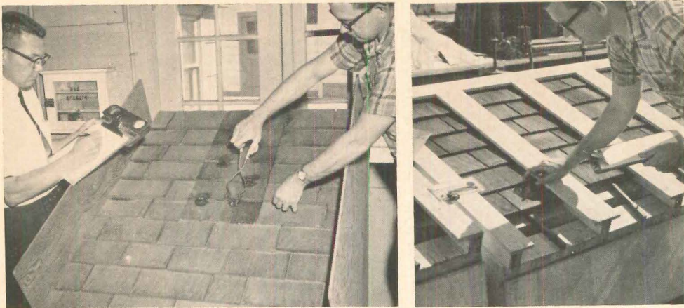
WOOD-SHINGLE FIRE TESTS include contact with burning brands (left) after exposure to sun and rain.
