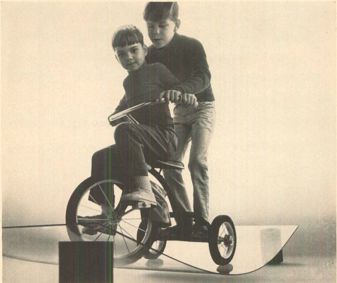
Two youngsters and a tricycle (150 lbs.) are easily supported by \frac{3}{16} " PPG Herculite K Tempered Safety Glass from a Safety Shield door.
