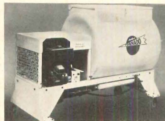
Multi-purpose sprayer is designed for textured coatings, waterproofing, concrete wall and ceiling coatings, and seamless-floor coating. Constructed with factory-built gear-reduction box and electric clutch. Delawanna, Clifton, N.J. Circle 242 on Reader Service card
