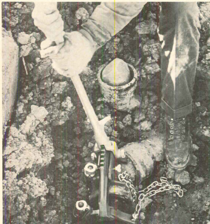
Soil-pipe assembly tool , for pipe using neoprene gaskets, works on elbows, Y's, T's, or straight lengths from 2" to 8" dia. Operator tightens chain around pipe and ratchets handle to draw pipe together. Ridge, Elyria, Ohio. Circle 225 on Reader Service card
