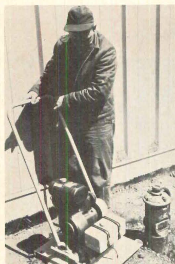
Vibratory compactor delivers 1700 lbs. of solid compaction per hr. over material layers up to 10" deep. Includes reversible shock-mounted guiding handle and idle control, to conserve fuel. With 4 h.p. gasoline engine. Wacker, Milwaukee. Circle 244 on Reader Service card
