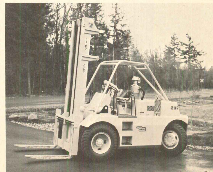
Forklift comes in capacities of 15,000, 16,500 and 18,000 lbs. There's a choice of oil clutch or automatic transmission and of gasoline, diesel or LPG power. Power steering, overhead and load guards are standard. Pettibone Mercury, Chicago. Circle 208 on Reader Service card
