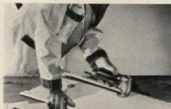
Electric hand shear cuts 20-gauge steel at a rate of more than 25' per minute. The shear permits left-hand cuts with 1/2" radius, right-hand cuts with 1" radius. Lumaside, Milwaukee. Circle 213 on Reader Service card
