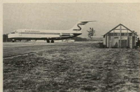
JET AIRLINER is positioned 100' from specially built test house alongside airport runway.
