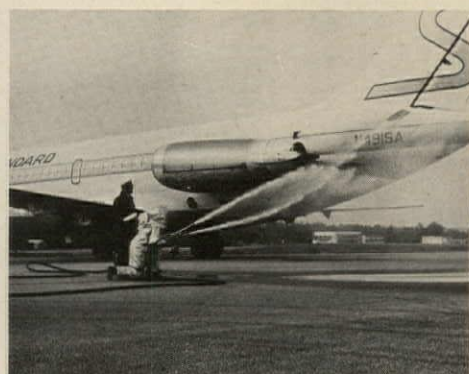
KNEELING FIREMEN aim firehoses into plane's jet stream to simulate heavy rains. Wind: 100 mph.
