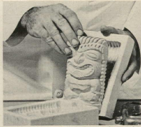
MOLD can be removed ten minutes after pouring. Metal, glass, wood or rubber molds may be used.
