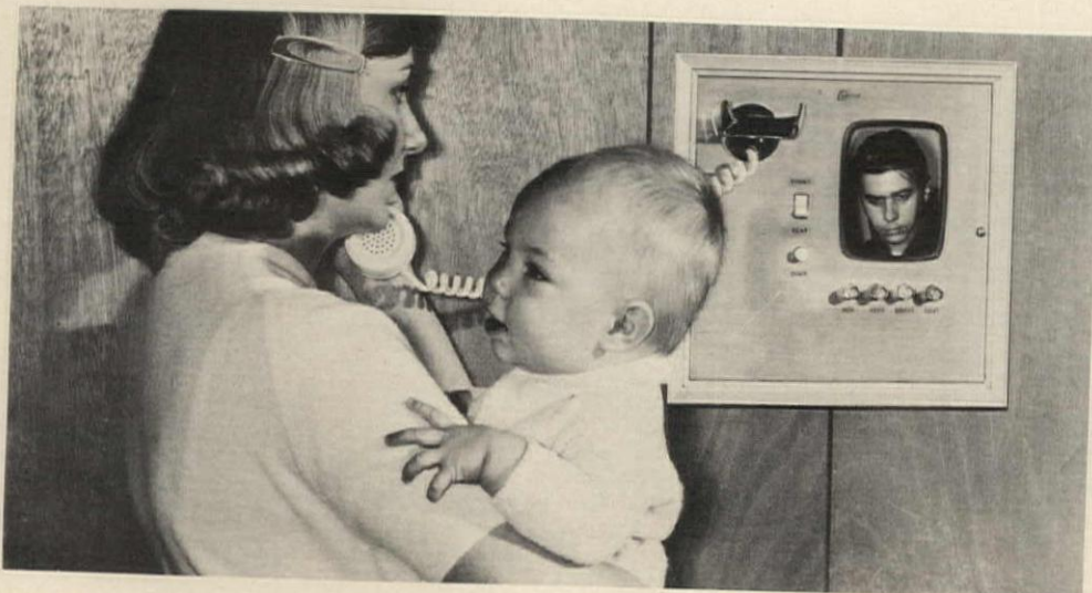
On-guard system is controlled by the doorman, who activates a door switch in the apartment door when the occupants go out. As long as the apartment remains on the system, anyone entering or leaving—by key or otherwise—will sound a constant alarm at the control panel (closeup, right). A red light identifies the apartment entered. Auth, Long Island City, N.Y. Circle 261 on Reader Service card
