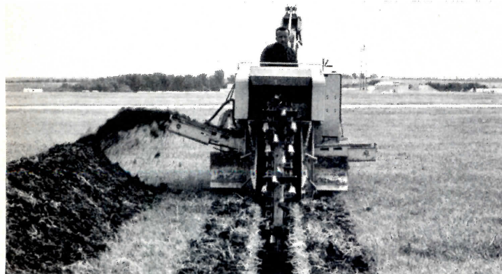
High-speed trencher has a double digging chain line and a high-capacity banana-shaped conveyor belt, will dig trenches from 2' wide to 5' deep at up to 1,500' per hour. The 60-hp unit has hydraulic controls. Davis Mfg., Wichita, Kans. Circle 324 on Reader Service card
