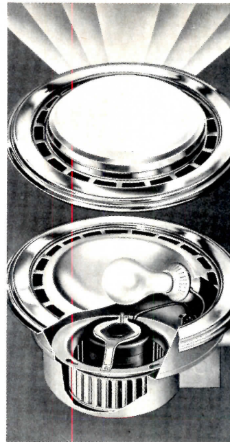
Combination fan/light for bathrooms can be wired for separate or simultaneous operation of vent fan and light. Blower motor floats on neoprene cushions, providing a low sound-level rating. The silver-anodized grille is 13 1/4" across and extends 2 1/8" below the ceiling. Adjustable brackets included. NuTone, Cincinnati, Ohio. Circle 349 on Reader Service card
