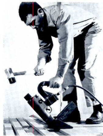
Floor stapler automatically positions and drives 1/2" 16-gauge staples in any thickness of hardwood flooring. Handle and shoe may be removed to convert tool to a conventional, trigger-operated stapler for sub-flooring, etc. Bostitch, East Greenwich, R. I. Circle 317 on Reader Service card
