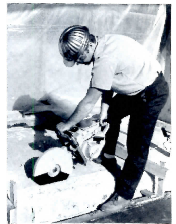
Portable saw has a self-contained 6 1/2-hp gas-powered motor, weighs 29 3/4 lbs and will cut through concrete, masonry and metal, wet or dry. A built-in governor assures constant cutting speed under all conditions. Robert G. Evans, Kansas City, Mo. Circle 318 on Reader Service card
