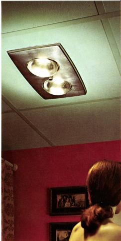
Radiant Heat-A-Vent® is ideal unit for apartments, motels, new homes. Instant heat from two 250w. Heat Lamps. Prewired for control of one or both lamps. Vents through 4" round duct. Installed quickly and economically. Also available: single-bulb Heat-A-Vent.
