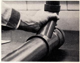
Installation is easy and fast. Joints are solvent welded, no threading. Stronger, too. PVC pipe weighs only a fraction as much as conventional materials, hence is easier to handle.
