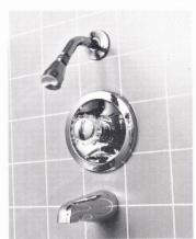
Nonscald faucet has just one moving part, balances pressure to maintain even water temperature despite drains on supply lines. Design features a single-handle control-either a dial, as shown, or a lever-in 14 styles. Delta, Taylor,
