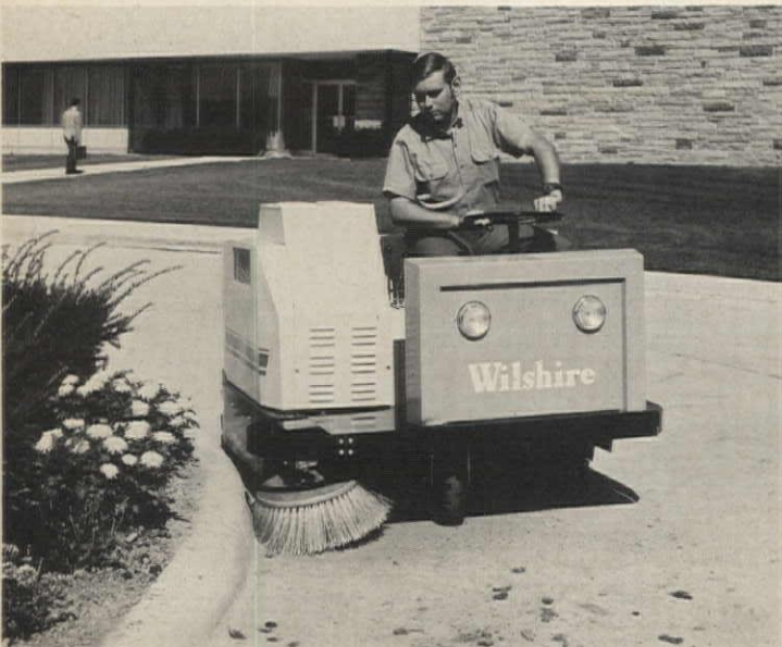
Power sweeper is equipped with hydrostatic transmission that lets operator use one pedal to go forward or backward. Main broom operates at a fixed rpm at any travel speed. Broom pressure is adjustable. American-Lincoln, Toledo, Ohio. Circle 230 on Reader Service card
