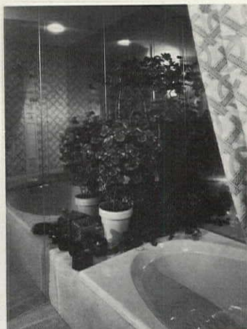
Stainless steel panels , at a cost competitive with fine wood paneling, are made of .025"-thick stainless laminated to ¾" pressed wood. Panels come 12", 24", 36", and 48" wide and up to 8' long,
