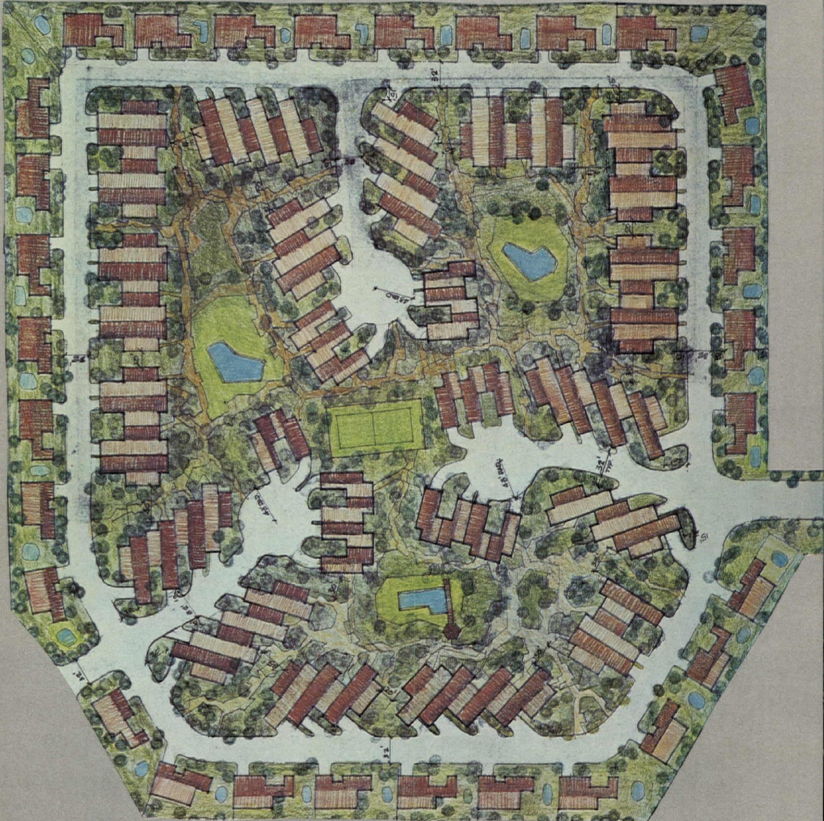
Site plan is divided into three phases, each with its own center green area and pool. First phase is at bottom, second phase, just completed, at upper right, third phase, just starting, at upper left. Detached units line the outside edge of the site, and a wall separates them from adjacent properties.
