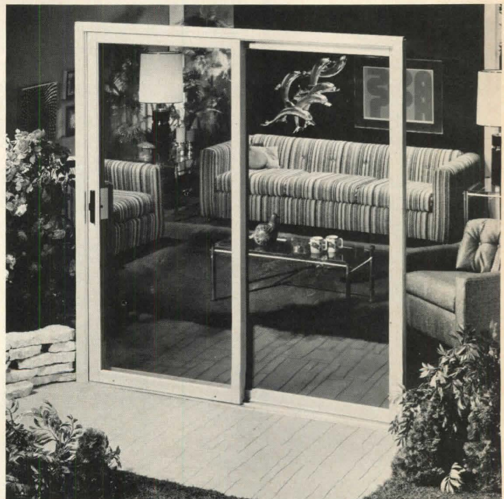
Wood patio door with insulating glass forms a tight wind and water-resistant seal. Movable panel is outside the fixed panel; when wind blows, the outside panel presses against fixed panel and frame to form the seal. Malta, Malta, Ohio. CIRCLE 278 ON READER SERVICE CARD
