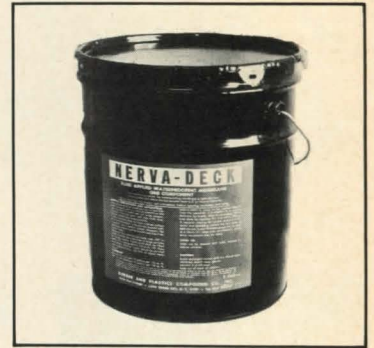
Waterproofing liquid, "Nerva-Deck," (above) is formulated from polyurethane rubber with coal tar additive. Applied with brush, roller or squeegee, liquid is fungi-, acid-, and alkaline-resistant. Rubber & Plastics, Long Island City, N.Y.
