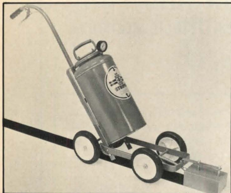
Economy model paint striper (above) can mark up to 120' per minute. The easy-to-operate unit is filled with paint and pumped until 20 lbs of pressure registers on the gauge. A trigger mechanism controls the flow of paint. Cooper Stanley, Denver. CIRCLE 262 ON READER SERVICE CARD
