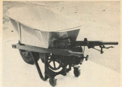
Gasoline-powered wheelbarrow (above) resembles a conventional unit in size and shape but can accommodate much heavier loads. Driven by a 3-hp, 2-cycle engine, the unit can handle up to 4 cu. ft. (600 lbs) of fresh concrete. Easy-to-operate thumb levers control motion and speed. National Concrete Machinery, Lancaster, Pa. CIRCLE 265 ON READER SERVICE CARD
