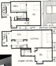
Largest multilevel shown in plan and photos, ha 1,650-sq.-ft. living Granite blocks (in ground at left) were used i original structure to counter balance cornices, and pro trude up to two feet into apart ments.
