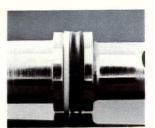
"Quad rings" are used as secondary seals, rather than "O-rings." Quad rings provide double sealing and because there is less friction, less wear.
