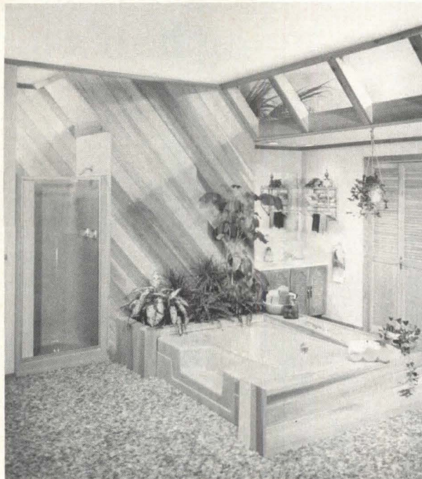
"Skymaster" skylights (above) consist of two layers of Eastman Uvex plastic sheeting separated by an insulating air space. Upper dome and lower diffuser sheet are electronically sealed. Tub-Master, Orlando, FL. Circle 207 on reader service card
