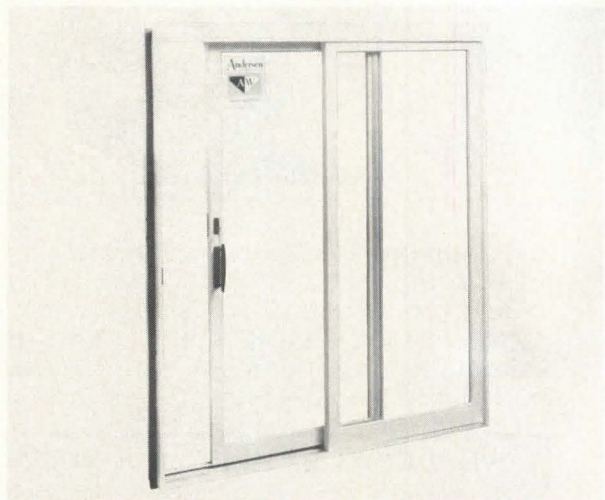
"Perma-Sheild II" sliding door (above) features low-maintenance vinyl sheathing over a preservative-treated wood frame. Double-pane safety insulating glass is standard. Andersen, Bayport, MN. Circle 208 on reader service card
