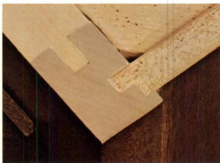
One-half inch thick end panels are lock jointed to frames. Wood corner blocks glued at all four corners.
