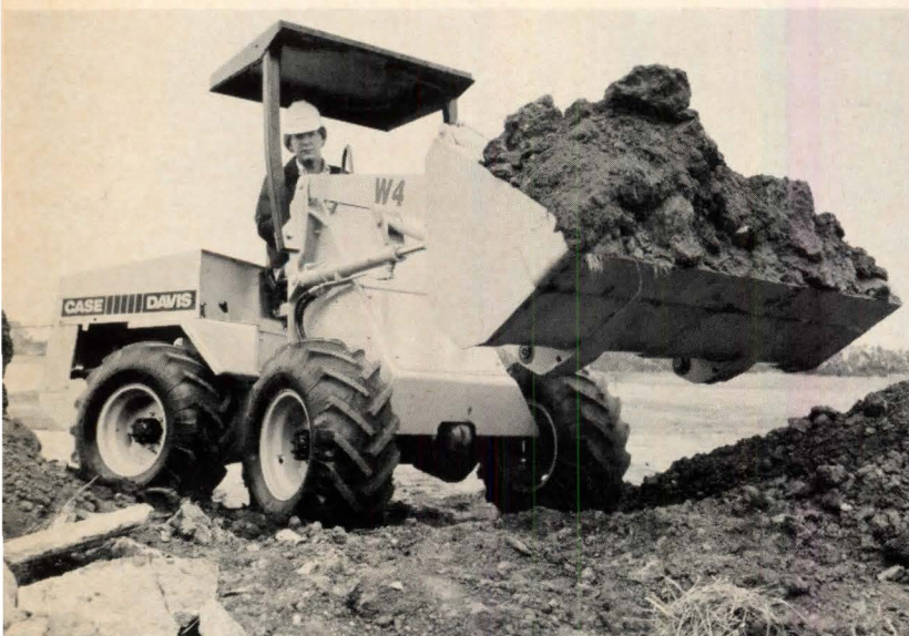
Articulated wheel loader, "Model W4" (above), is powered by a 35 hp, 4-cylinder liquid-cooled diesel engine. Unit features a mechanical self-leveling bucket. Davis, Wichita, KS. Circle 388 on reader service card
